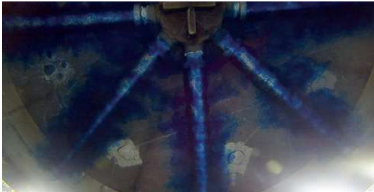
Blue dye tracer testing of a conventional radial fluid distributor, showing poor performance
