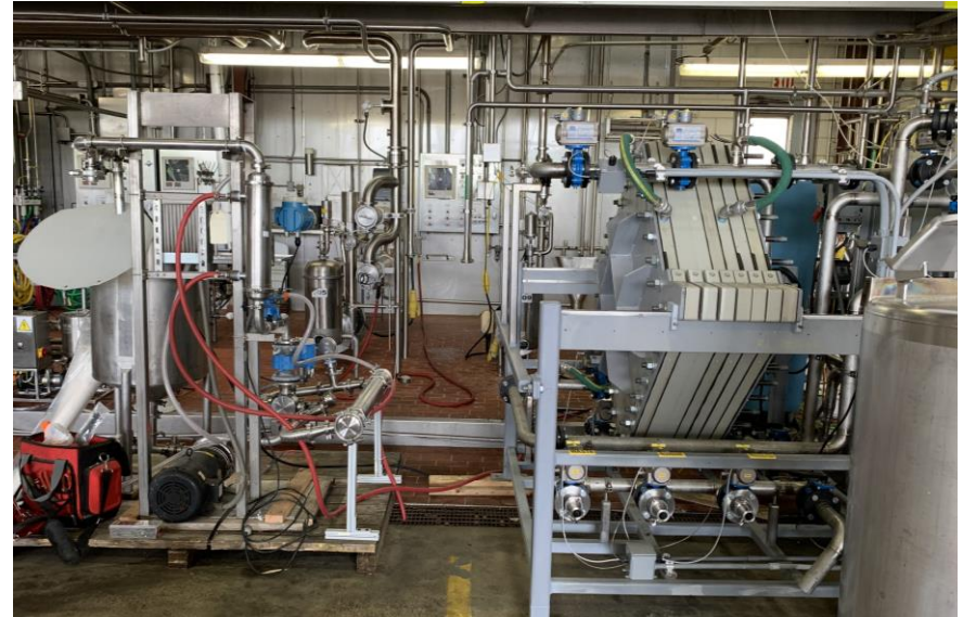
Testing in a U.S. dairy with a previous prototype Fractal Pack system
