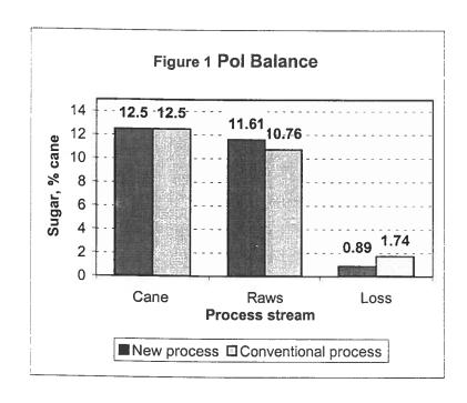
A pilot test program was carried out for several seasons at the Sugar Cane Growers Cooperative of Florida. Calculation of a material balance based on results of this pilot study shows an increase of 6.8 % in overall sugar mill recovery. The comparison of pol balance for conventional and the proposed process is presented by the graph in Figure 1. Breakdown of sugar losses throughout the mill shown in Figure 2, indicates that most sugar typically lost to molasses is recovered in the new process.
