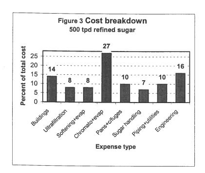
Understanding the cost structure of the process is of crucial importance for optimization. For our purpose we have factored the contribution of each unit operation into the overall capital cost of the new process (Figure 3). It is important to note that the calculations are based on initial rather conservative estimates.
